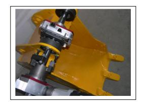
Optional: Facing attachment to machine thrust faces.
